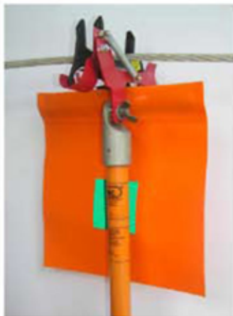
Open Snap Clamp being fitted with hotstick & Red Application Tool 1024
