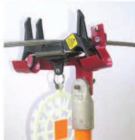
Fitting to overhead wires with application tool
