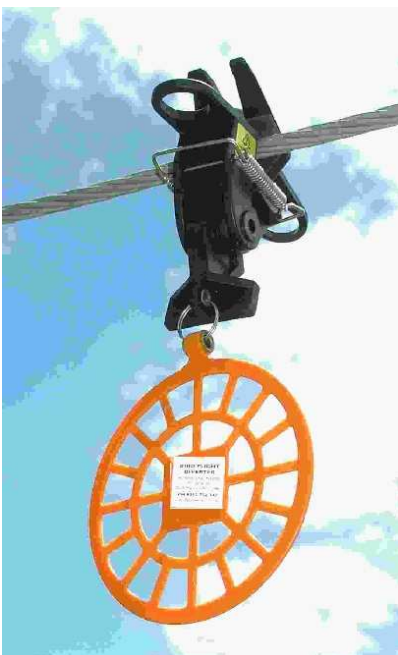
Bird diverter securely gripping the conductor
